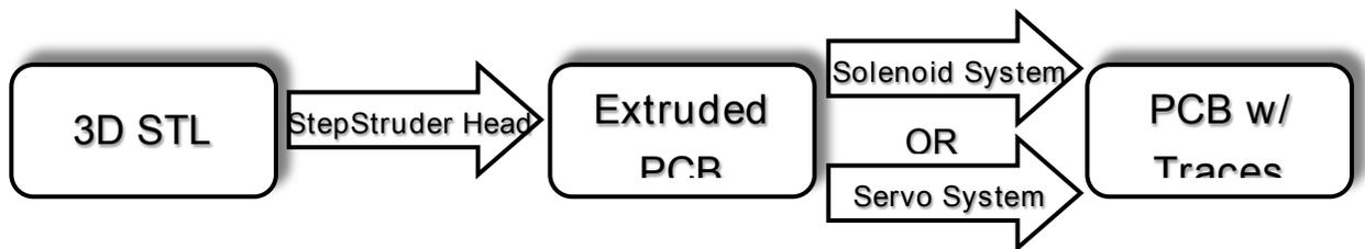
**3D PCB Creator Functional Block Diagram**
