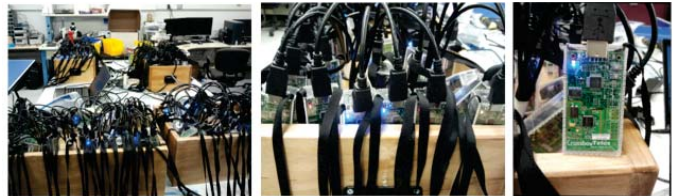
Fig. 3. TelosB nodes with base station and case. The TelosB was worn around the neck using an easy-break safety lanyard, though study subjects often complained about the total weight. A large 50-port USB base station connects the TelosB to a computer for programming and data download. The TelosB were dropped from our deployments due to complications in programming (only around 150 nodes of 200 actually enumerated, even using multiple USB buses), weight of nodes and base stations, and the non-rechargeable batteries.
