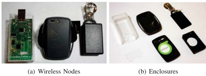
Fig. 2. Wireless nodes representing the three hardware iterations. From left to right: TelosB (Memsic), Irene (Moteware), and WREN (our design). They iteratively improve on size, weight, cost, and usability. Enclosures (b). Left: custom laser-cut acrylic case for the TelosB (3.55 cm x 2.54 cm x 7.11 cm). We used tape to hold the case together and to protect the wearer from sharp edges. Middle: standard Irene case. Right: the injection molded WREN case, making it smaller, safer, and more durable (3.3 cm x 1.52 cm x 5.33 cm).
