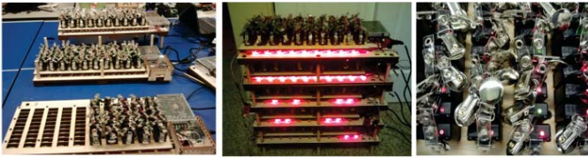
Fig. 5. Base stations with WREN nodes plugged in. We designed the base stations specifically for ease of use, storage, and maintenance in mind. The base stations can be stacked to save space. LEDs indicate the proper function of each blade and their status. The WREN features an RGB LED for debugging and as a status indicator for charging/fully charged while plugged in. These LED makes it simple to identify broken nodes, thus reducing the danger of re-deploying non-functioning systems.
