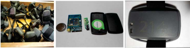
Fig. 4. Irene nodes with base station and case. After study subjects’ disapproval of lanyards, we designed wrist bands for the Irene nodes. The base station is the same as the TelosB with Micro USB instead of Female USB plugs. The Irene has a rechargeable Li+ battery, removing the need for replacing batteries. This made maintenance easier, but the high price and mechanical reliability issues didn’t allow us to scale beyond 200 nodes. Almost every USB connector on the charging circuits had to be epoxied due to breakage after several insertions.
